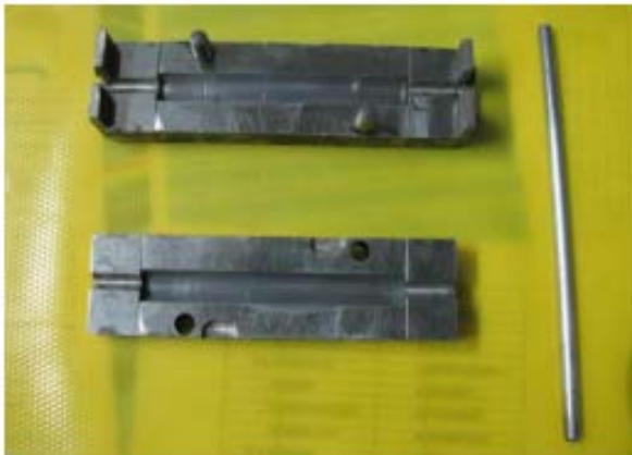
Mould used for Manufacturing Asymmetric Actuator
